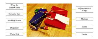
Fig. 13.3. Identifying the parts of the wafer seal device.
