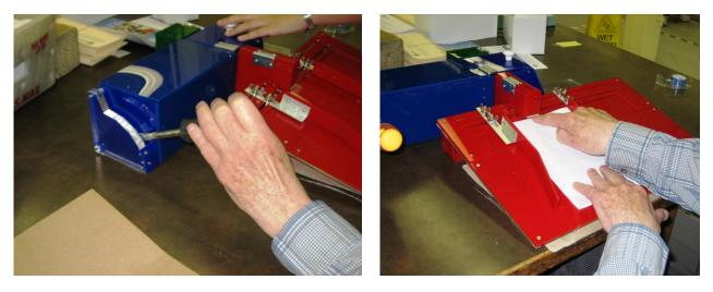
Fig. 13.4. The client is pulling the lever to dispense the next wafer seal, and then sticking the wafer seal onto the folded mailing.
