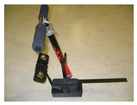
Fig. 13.9. Photo of the device. It mounts to the client's wheelchair by slipping the horizontal bar on the right side of the photo under the seat cushion. The client grabs the handles with both hands and pulls and releases the handlebar to count. The battery-powered circuitry is mounted in the black box at the bottom of the photo, and audio feedback is provided through the two speakers.
